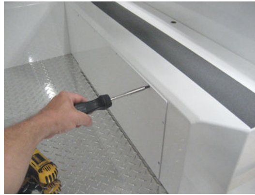
Attach seat cover plate with # 10 x 1/2" flat head sheet metal screws.
